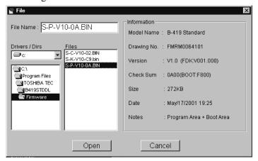
**7.** After highlighting the desired download file in the preceding screen display, click on **OPEN** and the screen display shown in the figure below will appear. Confirm the COM port conditions shown at the right of the screen.
